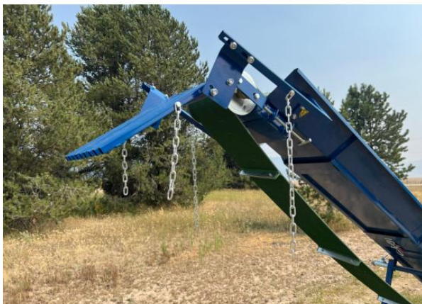
A Grizzly bars attached to the plates B Grizzly angle and discharge position
