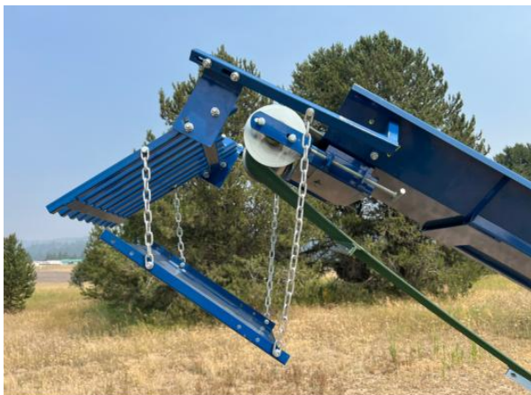
A Pan suspended below the grizzly bars B Pan angle and chain connections
