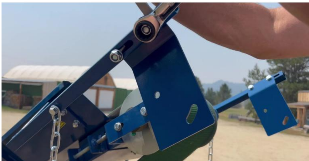
Left and right bracket plates mounted on the arms
