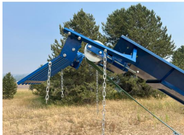
A Grizzly bars attached to the plates B Grizzly angle and discharge position
