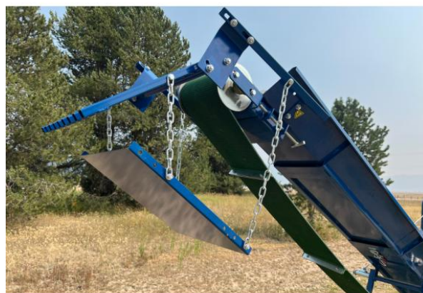
A Pan suspended below the grizzly bars B Pan angle and chain connections
