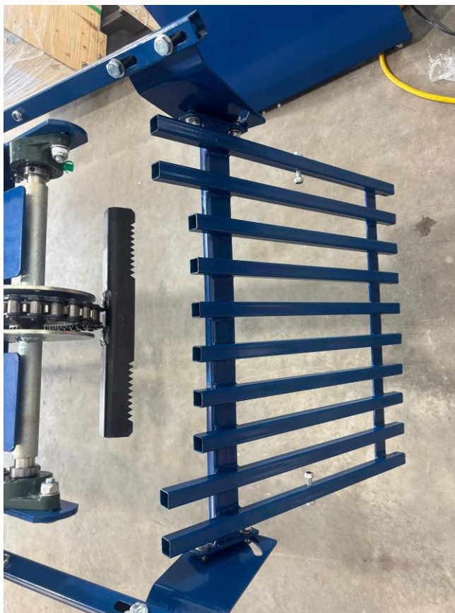
Grizzly-bar assembly attached between both swivel adapters
