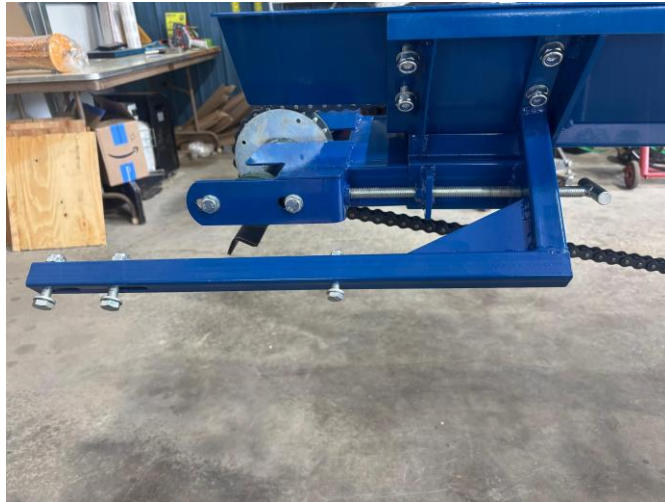
L-bracket secured using the rear side-extension bolts
