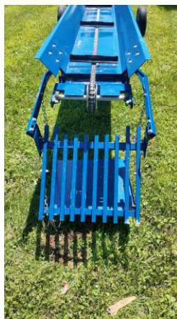
Completed RR2555 installation at the conveyor discharge end
