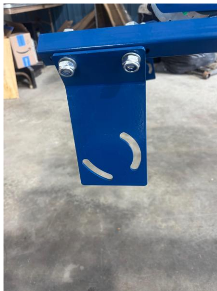
Slotted swivel adapter mounted to the L-bracket
