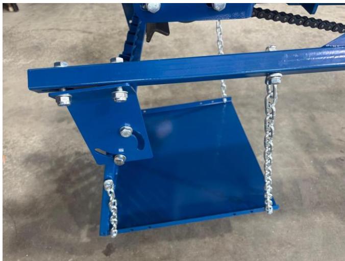
Grate pan suspended beneath the grizzly assembly
