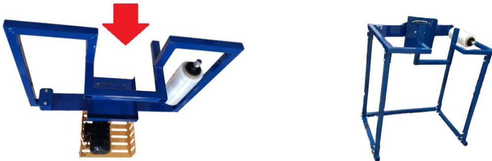
B Upper-frame opening faces upward C Upper assembly positioned on the legs
