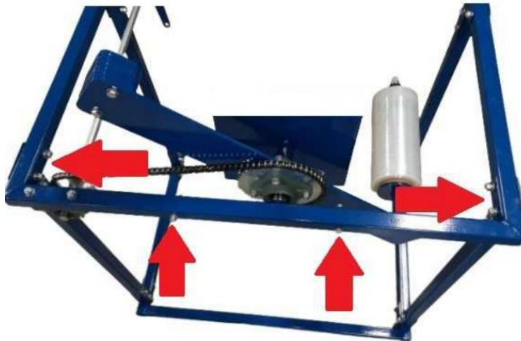
Guard-mounting fastener locations
