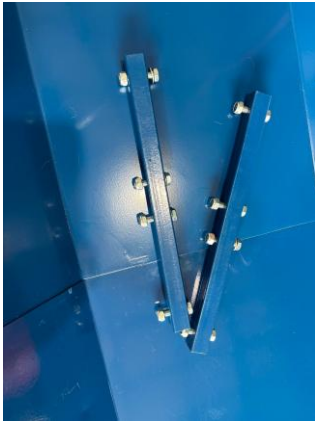
Position both trough frame supports
