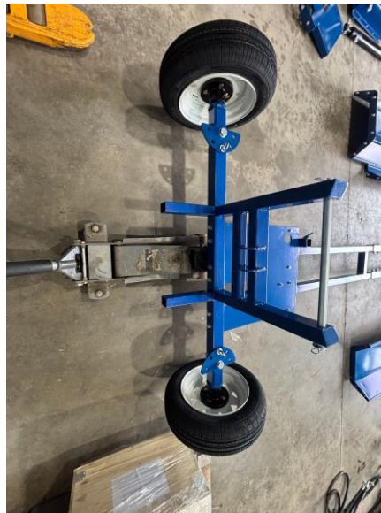
Both axle stubs and four-lug wheels installed
