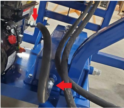
Pump suction hose connects to the pump side nearest the tank
