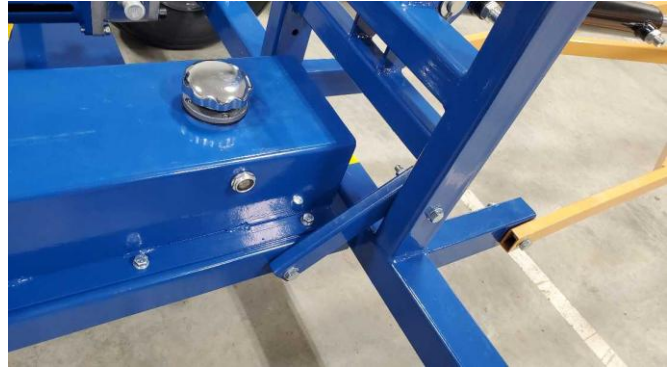
Frame-brace mounting position and bolt orientation
