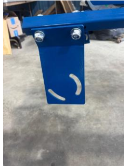
Slotted swivel adapter mounted to the L-bracket
