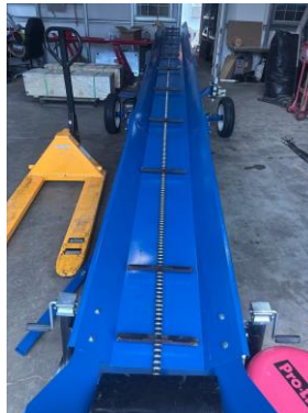
Joined trough seated on the support frame
