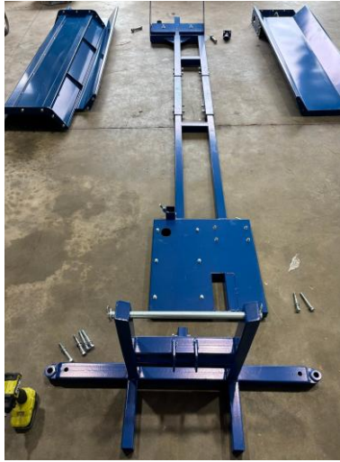
Lay out the base frame and conveyor trough sections
