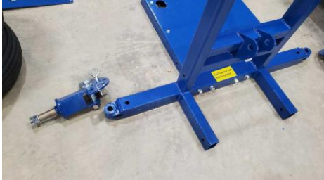
Position each axle stub at its swivel mount
