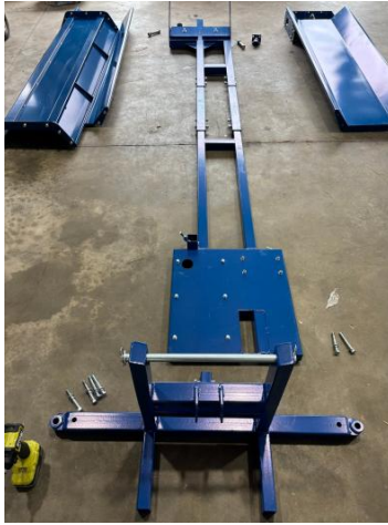
Base-frame sections arranged for assembly
