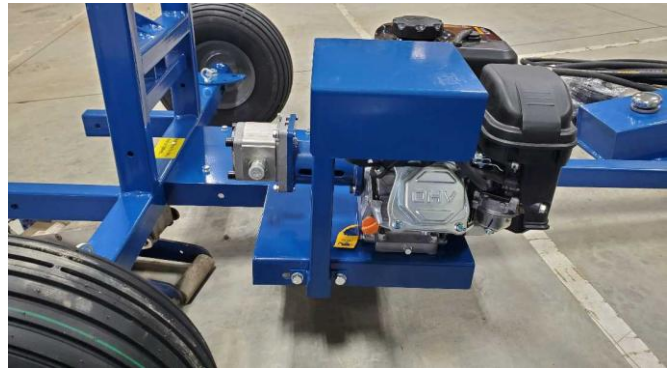
Protector installed beside the power unit
