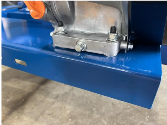
Raise the four mounting studs through the engine base
