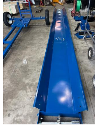
Four-section trough assembled on the ground
