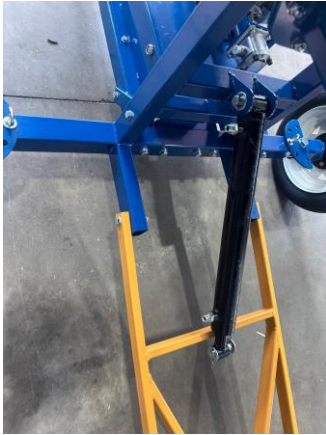
Lift cylinder and both blue frame braces installed
