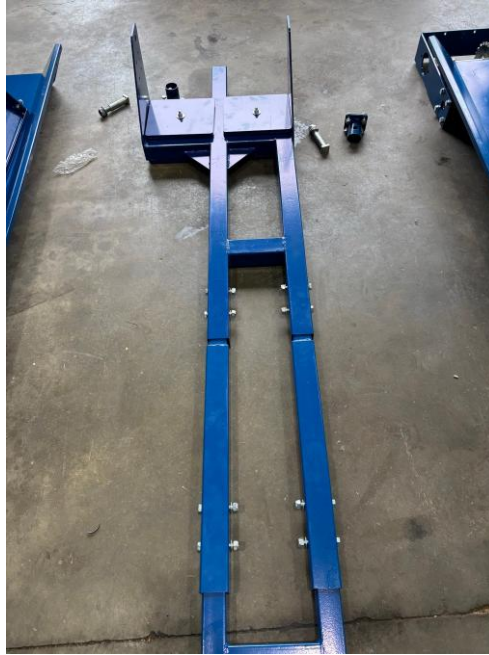
Front-frame orientation and connector locations
