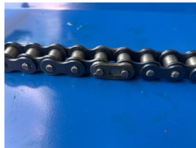
Master link used to join the conveyor chain
