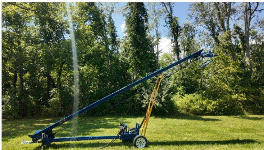
Completed RR510 shown in its raised operating configuration
