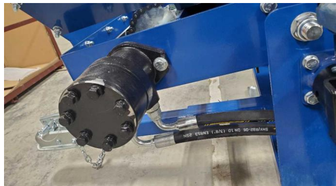
Motor-hose connections at the conveyor motor
