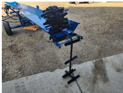
Conveyor chain before installation
