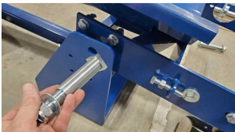
Identify the lower trough pivot fastener
