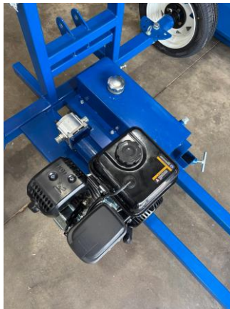
Hydraulic tank installed behind the engine and pump
