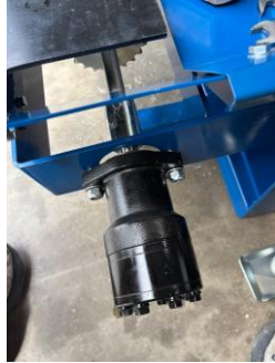
Hydraulic conveyor motor mounted at the lower trough end
