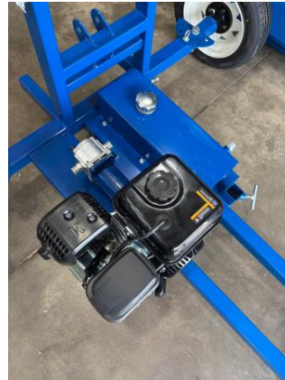
Engine, pump, and hydraulic tank orientation
