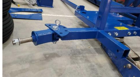
Tighten the swivel bolt without binding the pivot
