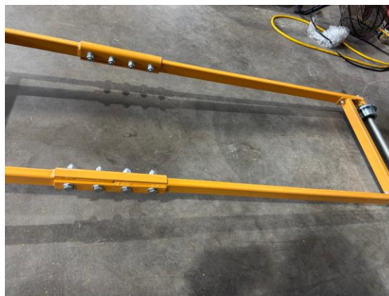
Four-bolt extension splice on each side
