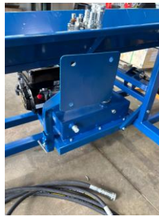
Control mounting plate and T-handle location
