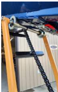
Route the chain through the raised conveyor
