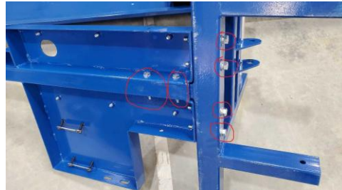
Install and tighten the remaining frame-joint fasteners
