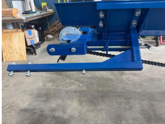
L-bracket mounted using the rear side-extension bolts
