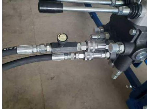
Needle valve in the upper cylinder hose
