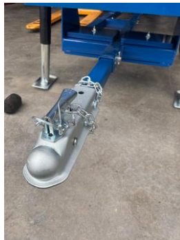
Front drawbar installed and pinned
