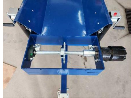
Drive-coupler alignment and motor mounting detail
