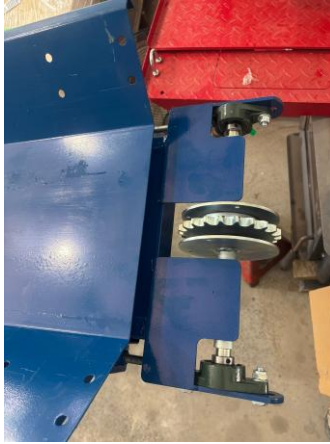
Upper roller and sprocket at the discharge end
