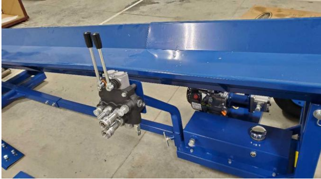
Right-side valve hoses for the lift cylinder
