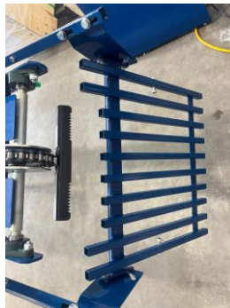
Grizzly-bar assembly attached to both swivel adapters
