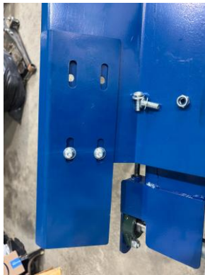
Discharge-end side extension and slotted mounting holes
