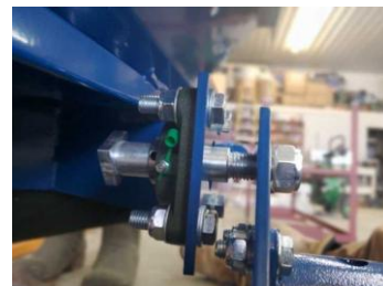
Lower trough pivot aligned and secured
