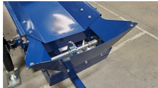
Motor-end plates fitted around the drive area
