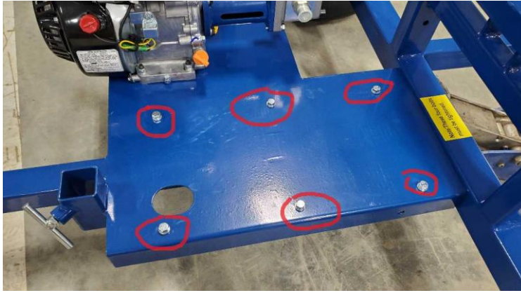
Remove the six tank-mount fasteners
