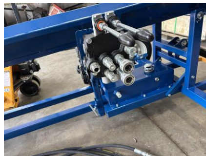
Control valve and operating levers installed
