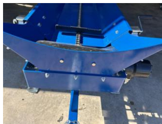
Optional rubber debris flap installed across the lower opening
