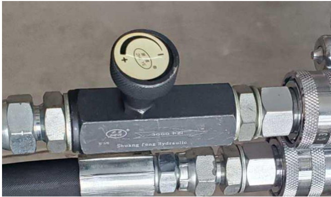
Needle valve used to control raising speed
