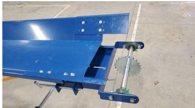
Both upper extensions installed around the roller assembly
