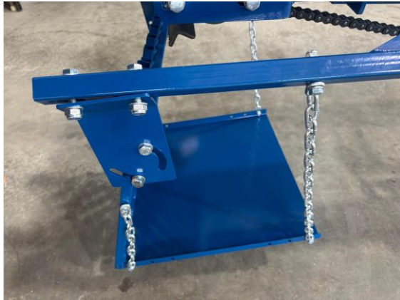
Grate pan suspended from the grizzly assembly
