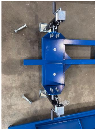
Both stabilizer jacks installed
