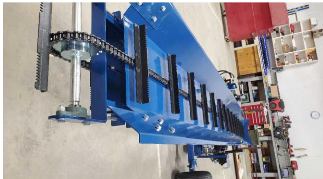
Chain routed through the trough
