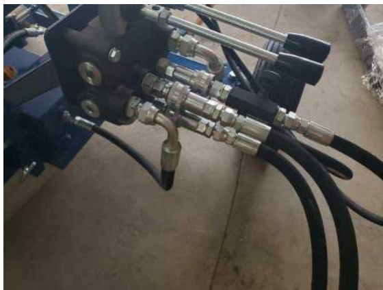
Pressure hose routed to the control valve
