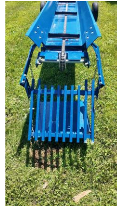
Completed grizzly bars and grate pan
