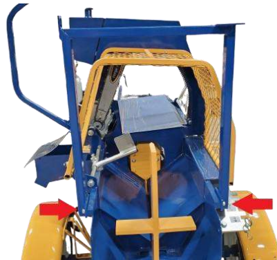
Tower fastened to the end of the EcoPro200
