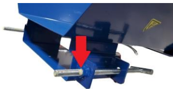
Lubricate both adjuster threads
