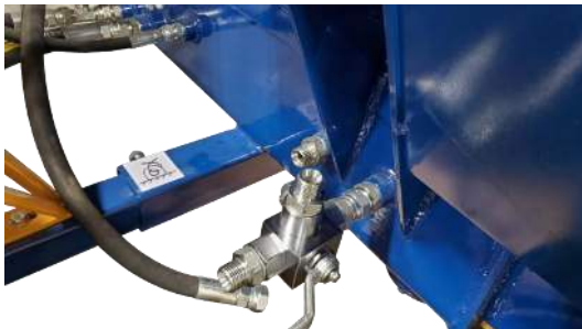
Original hose and reservoir plug removed
