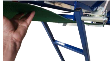
Belt clearing the support-stand center crossbar
