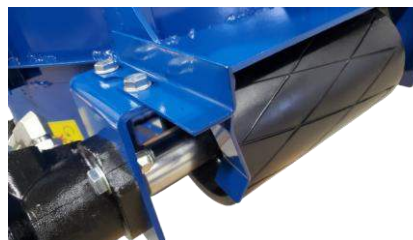
Belt guide positioned at the motor end
