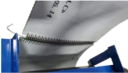
Adjust both tension bolts in equal increments
