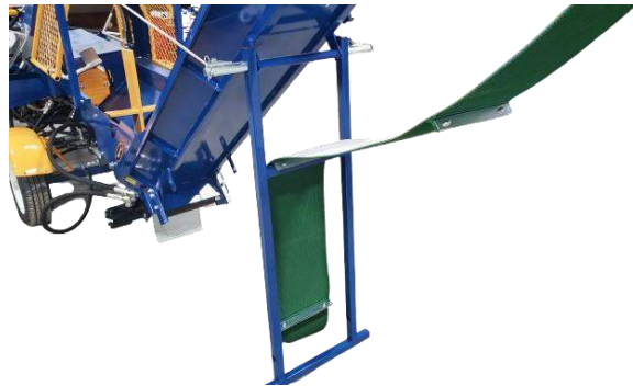
Belt routed through the stand above the center crossbar
