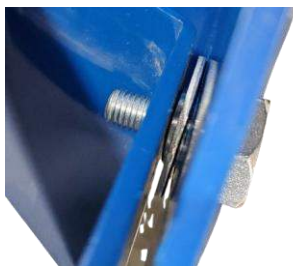
Washer placed between the machine bracket and conveyor tab
