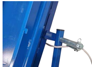
Washer and retaining pin installed
