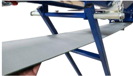
Keep the end roller square with the conveyor frame
