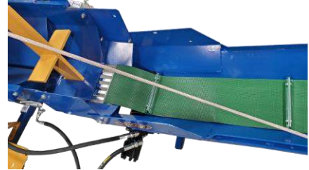
Belt routed around the motor roller
