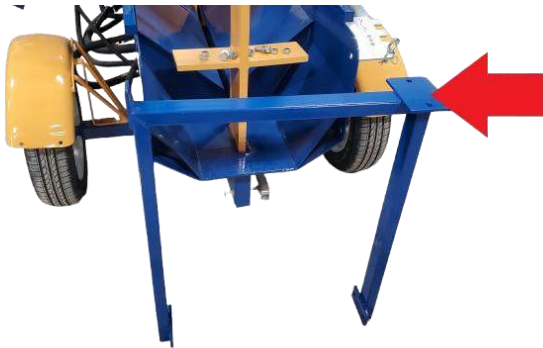
Winch mounting plate oriented toward the operator side
