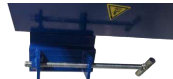
Adjuster backed out near the end of its travel
