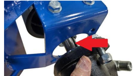
Motor shaft key aligned with the coupler keyway
