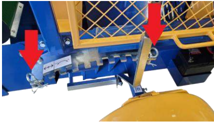
Folded conveyor raised into the secured position
