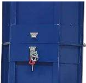
Safety latch installed
