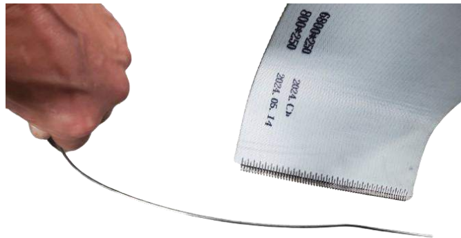
Hinge pin removed from the belt lacing
