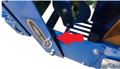
Belt-retaining bar installed
