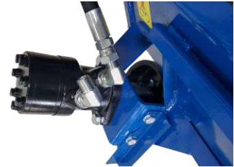
Hose route between the EcoPro200 and conveyor motor
