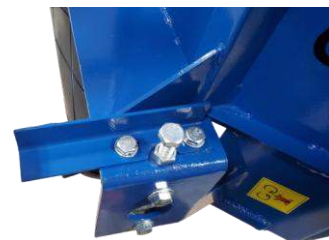
Belt guides installed
