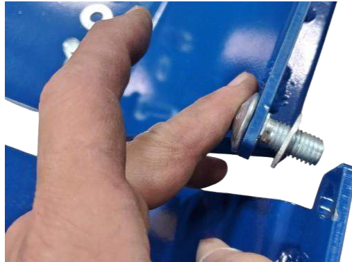
Upper section aligned at the folding joint
