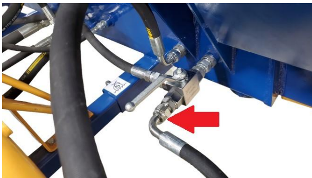
Second hose: 90-degree end connected at the control valve
