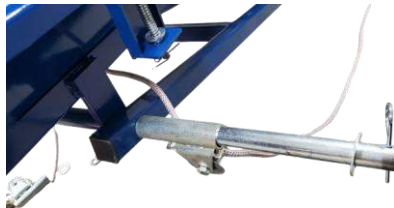
Rod passing through the stand and conveyor frame
