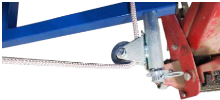
Cable seated over the first roller
