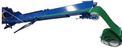
Belt started along the conveyor trough
