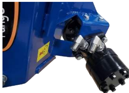
Motor installed with hydraulic fittings facing upward
