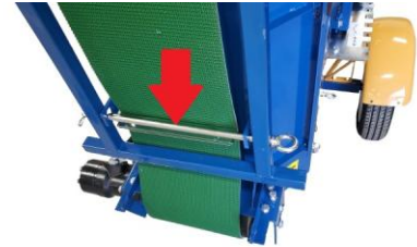
Both safety pins securing the conveyor to the frame
