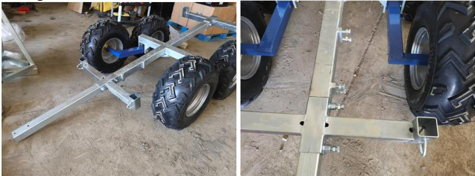
8.) Slide the cage over the inner frame rail. Installed right up against front frame portion. Install 2 large bolts and tighten.
