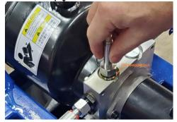
6) When you pull the housing out you will see the stainless steel screen that needs cleaned, use brake cleaner or degreaser and a brush to clean the screen out. Screen can be removed if necessary for cleaning.
