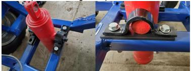
15.) Install hydraulic pump-there are two short, gold colored bolts that came in the same box as the hydraulic pump unit.
