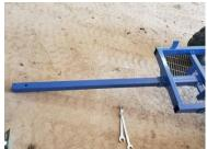
9.) The large bolt installs through frame tube and main frame, tighten nut. Tighten 2 bolts on the side of the frame rail, and then tighten retaining nuts.
