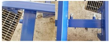
10.) Slide battery box onto frame tube and then slide the tongue jack on.
