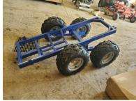
8.) Install frame tube into main frame, ensure the holes at coupler end face up & down.
