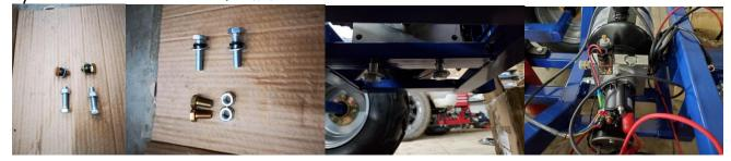
16.) Install hydraulic hose, mount to pump and cylinder, use tabs on frame and the supplied zip-ties to hold the hose to the frame. Cylinder can be mounted with the fitting either way as shown in the photo below
