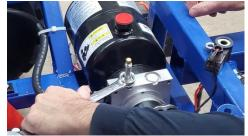
5) When oil starts to seep out of the threads, stop turning until there is no pressure left in the oil coming out, usually just a few seconds.
