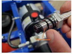
7) Re-install housing with clean filter using 15/16 wrench.
