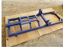
3.) Place the walking beams between the tabs on either side, there is not a right or left, either walking beam can be used for both sides, however the longer part of the arm goes to the front, line up the hole in the walking beam with the tabs on the frame, push pin in to hold axles in place.
