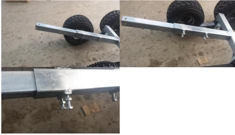
11.) Frame rail should extend approximately 40" passed main frame, tighten all 4 bolts and then all 4 nuts.
