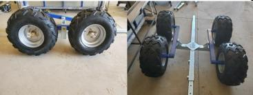
9.) Flip frame section over so that the frame is higher than the walking beams and slide frame rail in.
