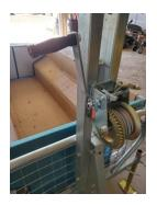
26.) Remove bolt and reverse the position of the swivel lock pin.
