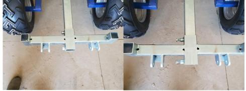
13.) Find front bunk frame and slide onto the frame.
