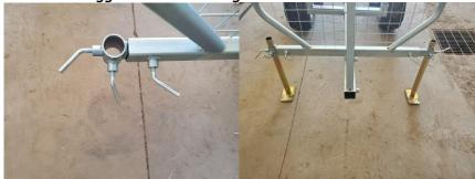
17.) Find hitch swivel and install to front of frame tube, tighten bolts, grease swivel with grease gun.
