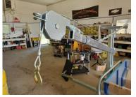
36.) Connect winch line hook to loop inside of tub.
