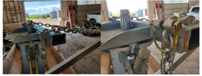
33.) Tighten bolt holding chains to boom.
