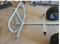
16.) Install outriggers and retaining handles.
