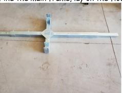
4.) Place the walking beams between the tabs on either side, there is not a right or left, either walking beam can be used for both sides and insert pins.
