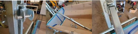
31.) Remove chain locking pins from swivel plate.
