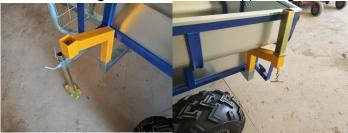
Test winch position, when lifting the tub winch line must not tough tub end door.
