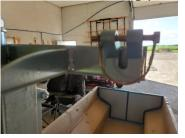
32.) Lift crane arm to desired position, run chains into locks on the swivel plate, install lock pins,
