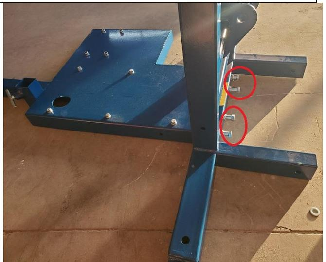
Lift the frame up and insert the 2 -16mm bolts with the 17mm nuts, tighten these and then tighten the 4 - 16mm bolts in the red circle as well.
