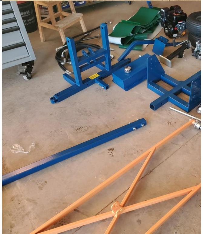
Find the frame section that the hydraulic tank will mount to and the frame section that the wheel will mount to, remove the 6 - 16mm bolts.
