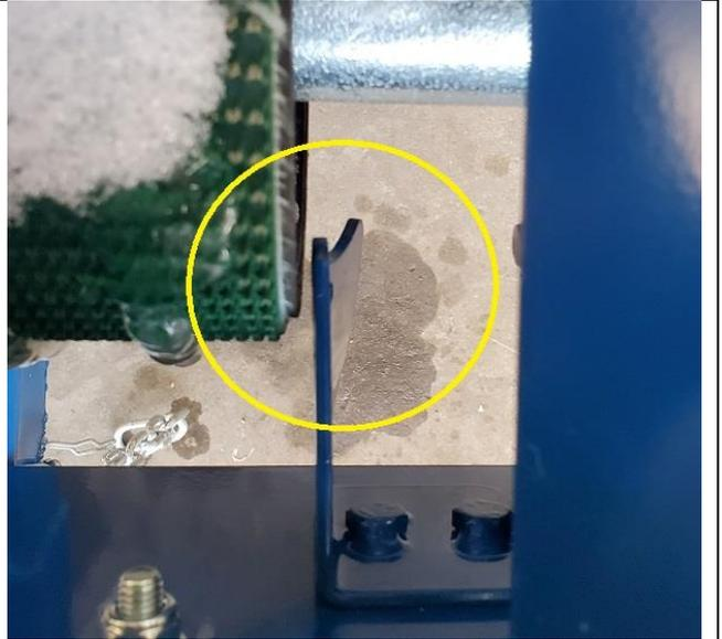
Mount the 2 side plates and tighten all the bolts.
