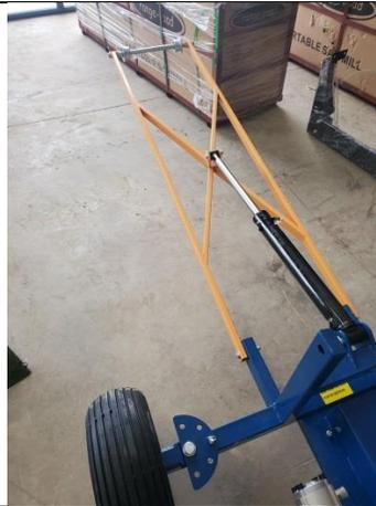
Insert the round pin into the upright tabs and secure in place with pins supplied.
