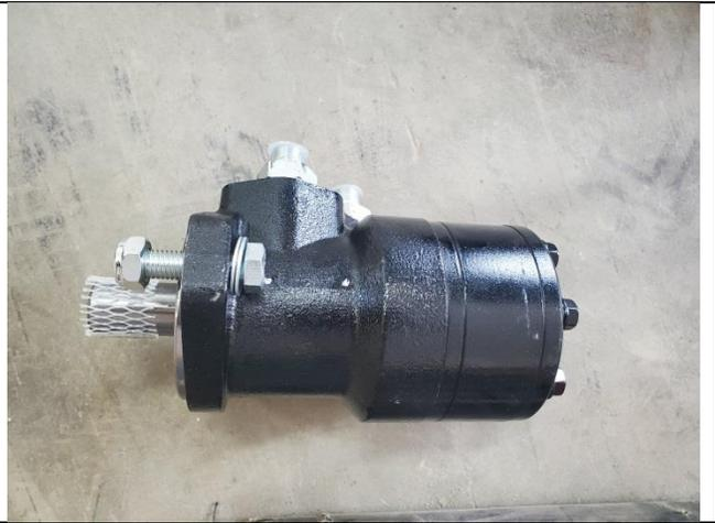
Tighten the 16mm Bolt x 17mm nut, tighten both allan keys on the coupler.
