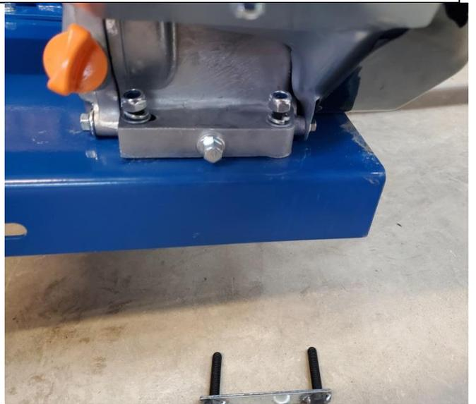
Once all 4 - 13mm nuts are threaded on, tighten them securing the engine into place.
