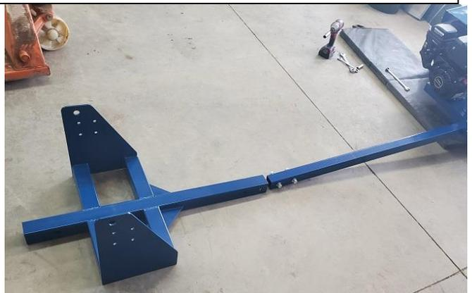
Remove the 2 - 16mm bolts x 17mm nuts, line up the holes in the 2 frame sections, reinstall the 2 bolts and nuts and tighten.
