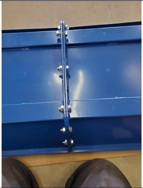
Find the rear cross frame that the cylinder attaches to and mount to the stubs on the frame behind the wheels. The 2 bolts must be loose enough so that the frame can move up and down without binding.
