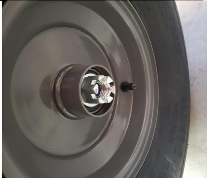
Put in the cotter pin and bend it so it will not interfere with the cap.
