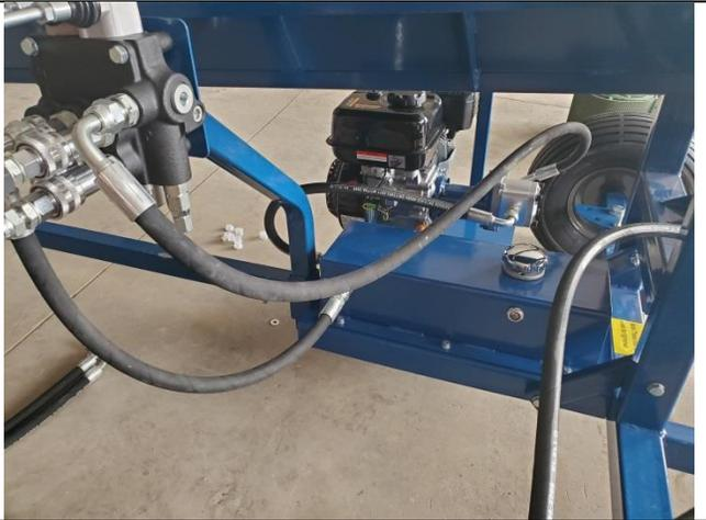
Plug the conveyor motor hoses into the control valve using the quick connect fittings.
