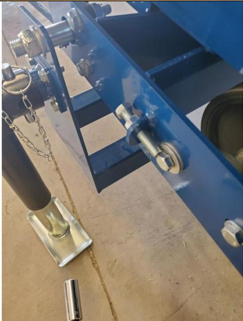
Adjust the T handle until the measurement is the same on both sides.
