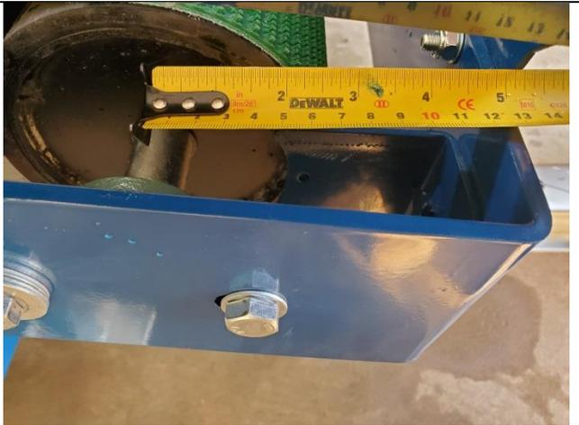
Use the adjuster bolt to make the measurement the same on both sides. Now the bottom roller should be square.
