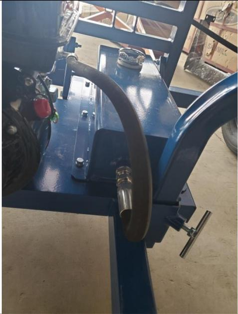
Install the pressure hose from the pump to the control valve,
